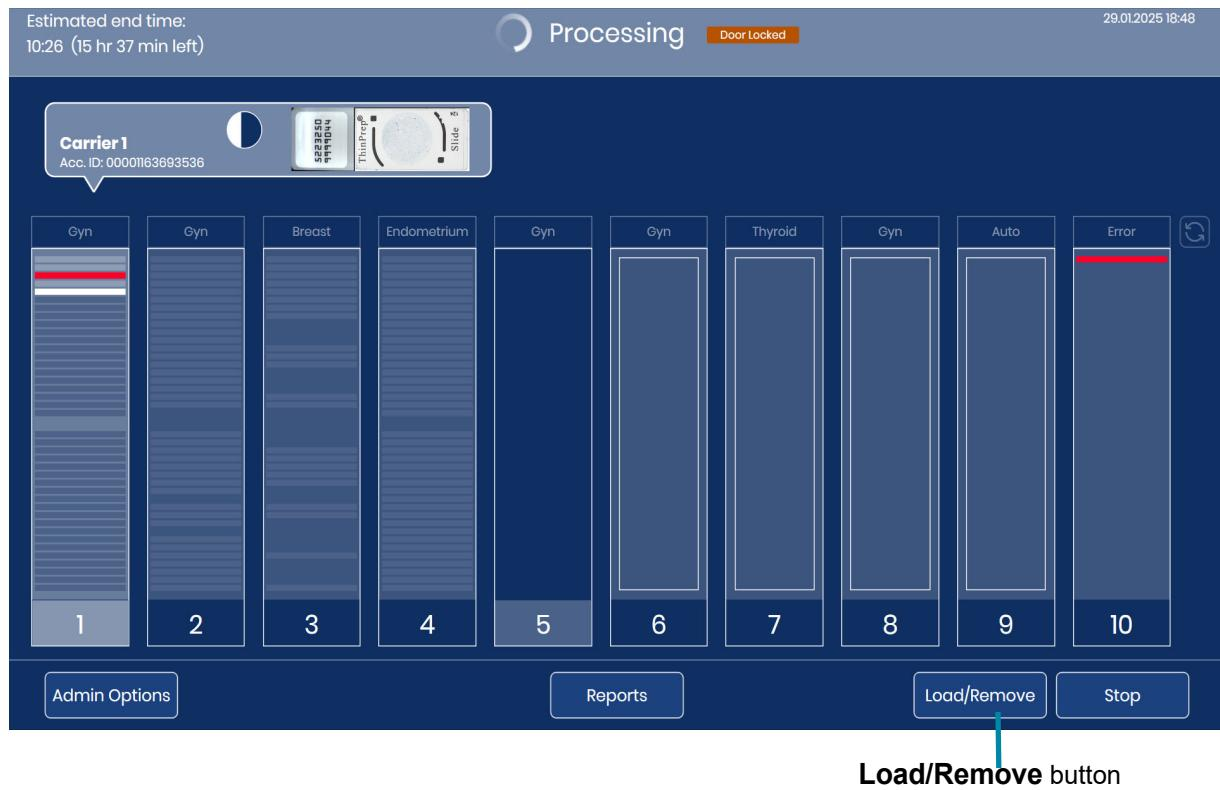
**Figure 1-4-17 Slide processing: Load/Remove button**
