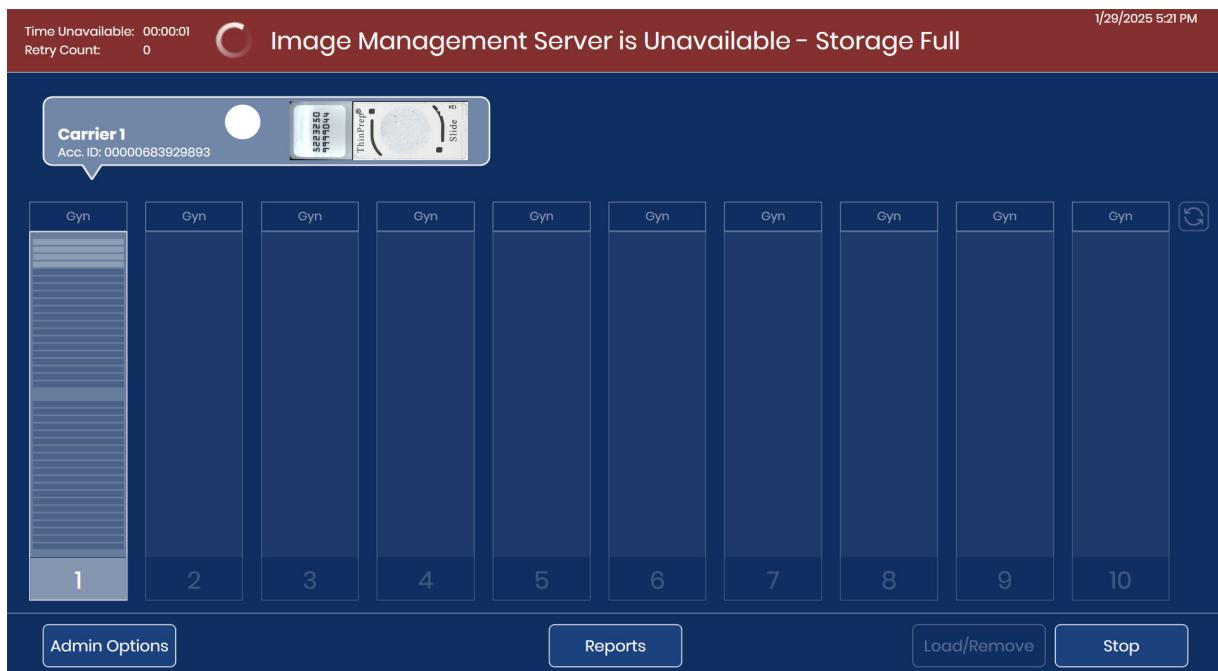
**Figure 1-6-2 Insufficient storage available on the Image Management Server**
